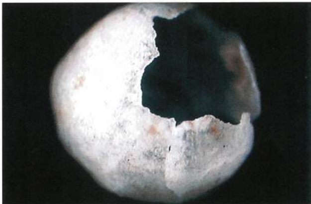
Membrane decomposed by 12Months exposure to sunlight /Meister SS
